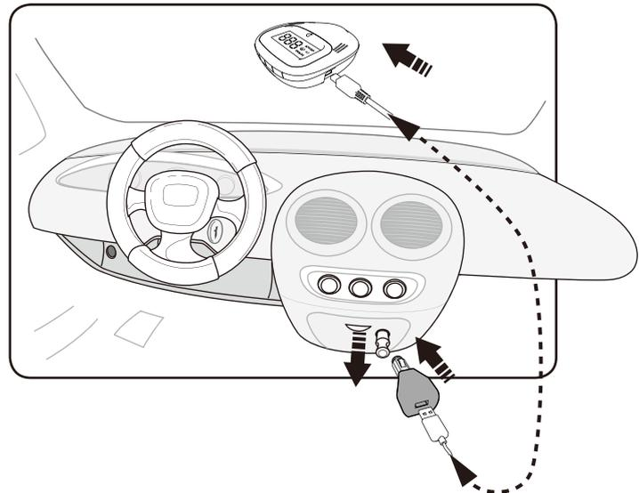
1. Connect the power cable with the plug.
